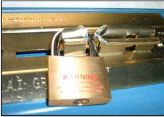
Faced with a high-security padlock, a thief can still cut around the latch of a standard self-storage slide bolt.
